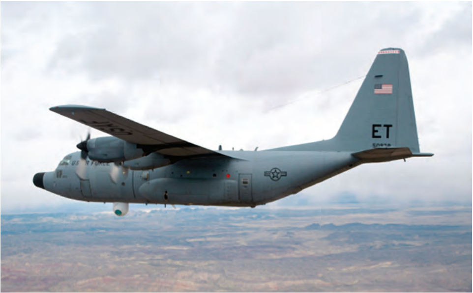
FIGURE 8. NC-130H TEST AIRCRAFT WITH THE ADVANCED TACTICAL LASER
