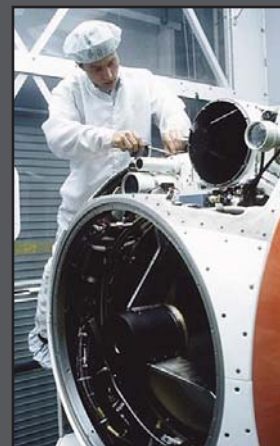
This image shows a technician working on the optical telescope turret of the ALL HEL weapon. Note the array of ancillary optical sensors (USAF).
