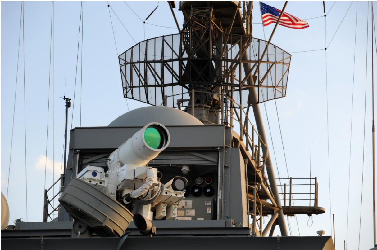
Figure 3 – The AN/SEQ-3 aboard the USS Ponce, able to mitigate threats from missiles, artillery and rockets.
