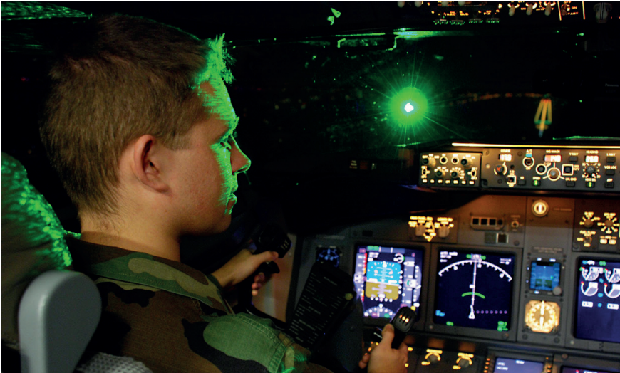
Figure 6. Cockpit windows and air/spacecraft optical sensor functioning may be dazzled by low-power lasers. 19
