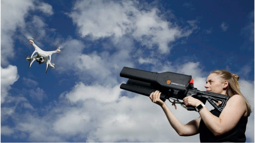
Figure 7. Example of “front door” electronic attack to disrupt the control signals between the drone and its remotely located controller. 21
