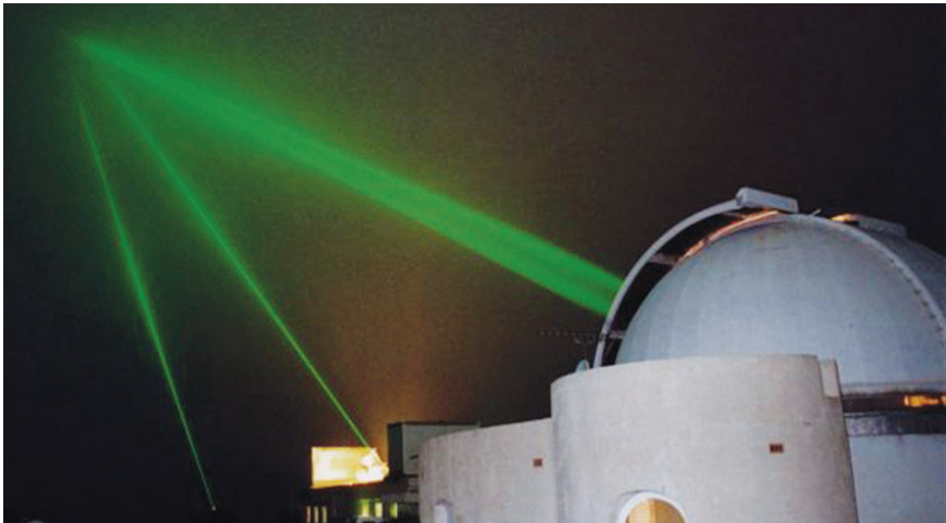
Figure 28. Laser energy has been reflected from reflectors mounted on artificial objects left on the Moon surface by the NASA Apollo program. 80
