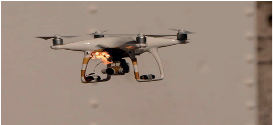
Figure 5. Laser thermal damaged drone target. 18
