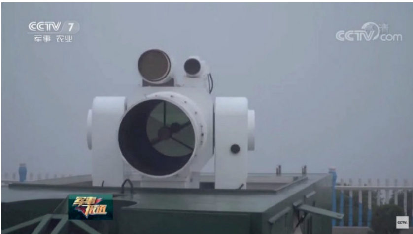
Figure 18. Chinese media has reported that the People's Liberation Army Navy is testing a prototype HEL DEW (displaying possible beam director, target tracker, and rangefinder). 58
