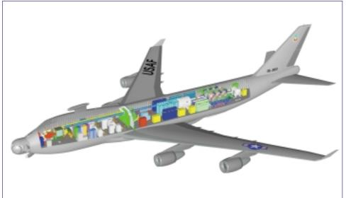
Construction of the Airborne Laser entails integration of several complex subsystems on a commercial airframe.
